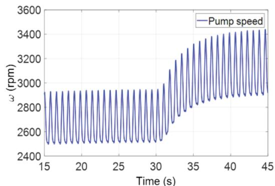
Fig. 14. Time waveform of pump speed at the transition from rest to exercise
