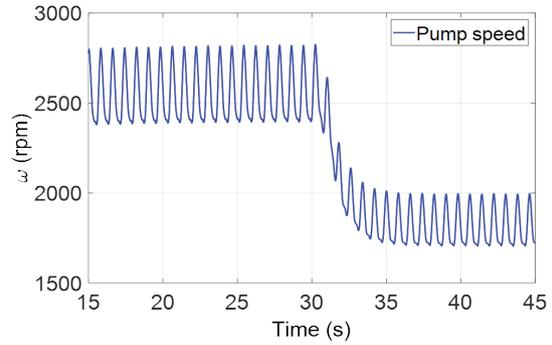
Fig. 10. Time waveform of pump speed @ the transition from normal to rest
