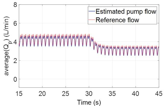
Fig. 11. Estimated pump flow vs Reference flow @ the transition from normal to rest
