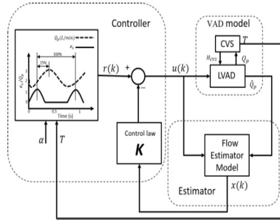
Fig. 5. Block diagram of the human cardiovascular system in combination with the controller, estimator, and reference input.
