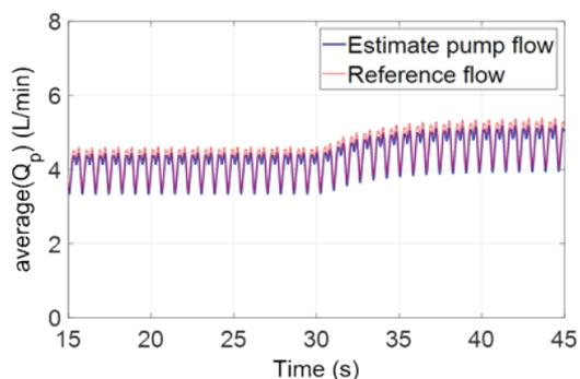
Fig. 15. Estimated pump flow vs Reference flow at the transition from rest to exercise
