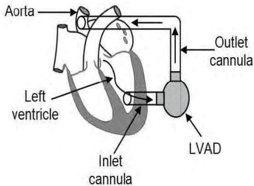
Fig. 1. Schematic diagram of the left ventricular assist device connected with the human heart.
