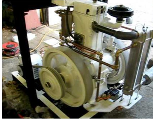
Fig. 2: Photo Image Diesel Engine with Electric Generator
