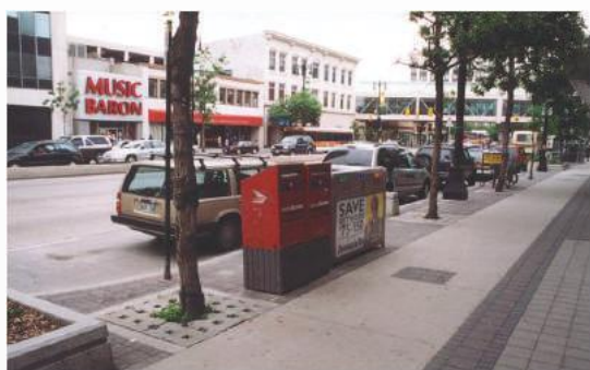
Figure 80: Street Furniture Street furniture located out of accessible route.
