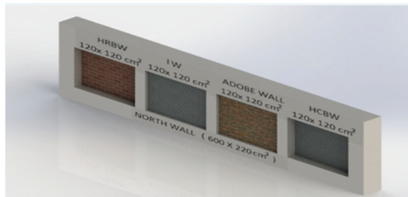
Fig.2 The four building wall systems separated by siporex layer
