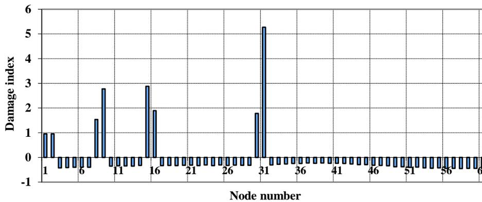
Fig. 9. Damage indices of ULS curvatures of *Case 6* of damage
