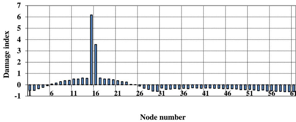
Fig. 6. Damage indices of mode shape curvature of Case 3 of damage
