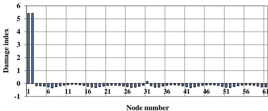
Fig. 4. Damage indices of mode shape curvature of *Case 1* of damage
