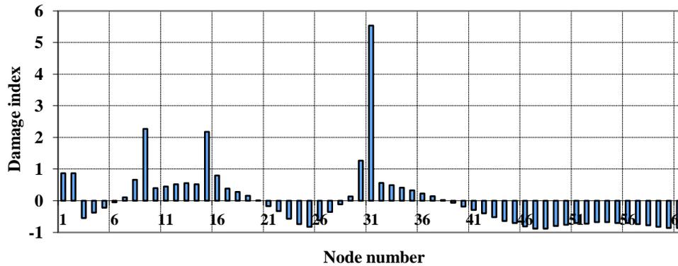
Fig. 8. Damage indices of mode shape curvature of *Case 6* of damage
