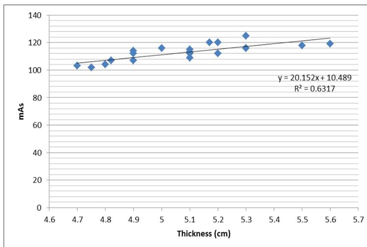
Figure 1. Correlation between the compressed breast thickness and tube current rate (mAs) for Craniocaudal projection  $60^\circ$  film (p<0.01)
